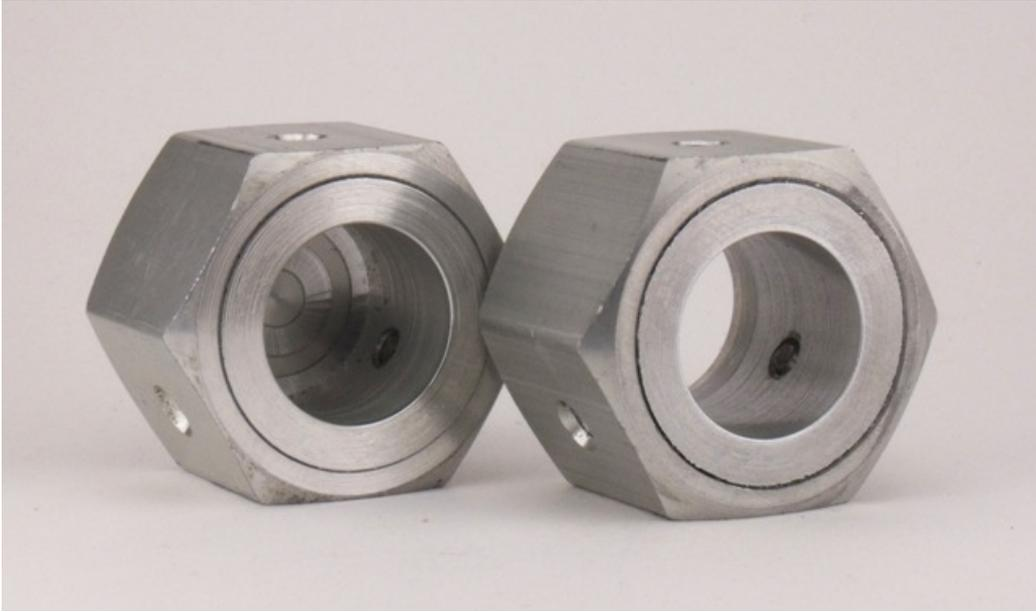
The nuts are simply hexagons with a hole through the middle. One of them in the picture is closed on one side but I have since bored the hole all the way through.
