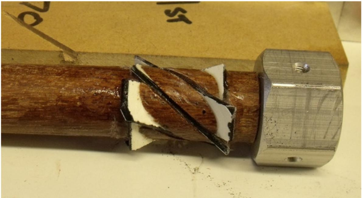
To keep all my cuts uniform around the blank I just used an end stop on the chopsaw.
