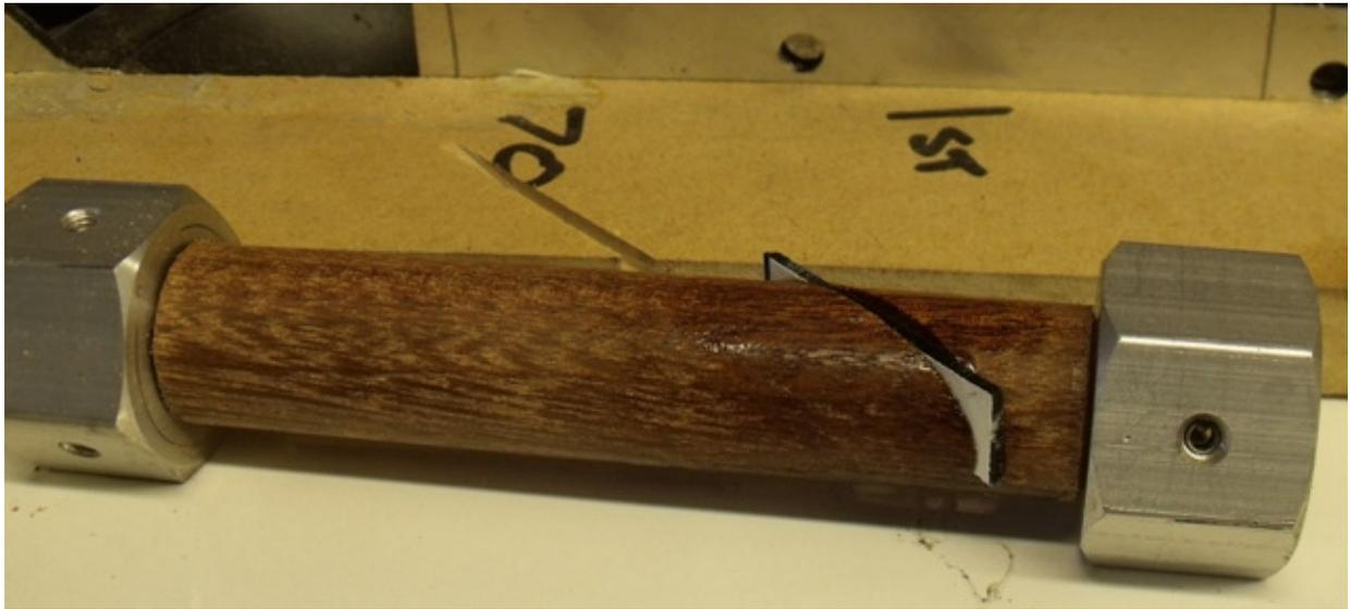
Above is the first cut with an insert already glued in. You will need to make sure that the insert isn't wider than the nuts or the flats of the nuts won't sit flat on the cutting tool table.
