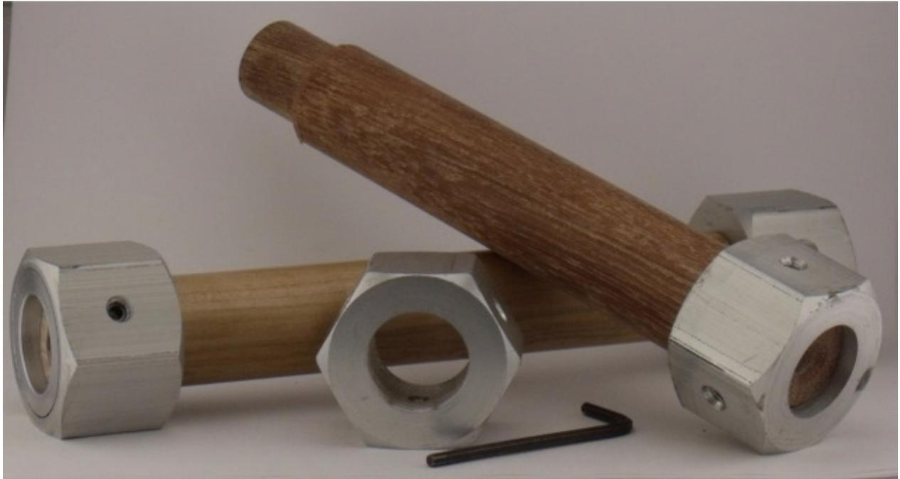
In the above example, two blanks were rounded between centres and then the ends turned down so they fitted in the holes.
