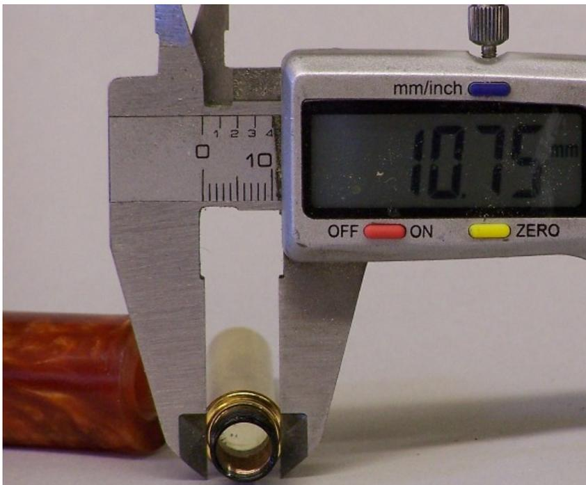
The tool handle will need a hole all the way through, the same size as the bolt diameter. One end of the handle will need a bigger hole to bear against the trim ring
