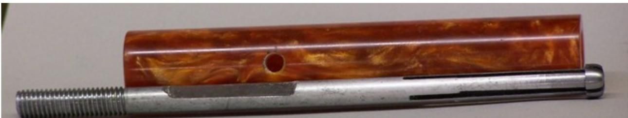
Here is the handle cut to length. Note the tapped hole in the side. This is just for the knob to stop the bolt from rotating while you extract the coupler. Also note that the flat is long enough for the bolt to travel the required distance at least
